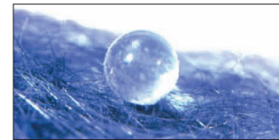
Cryogel Z and Pyrogel XT are super-hydrophobic
